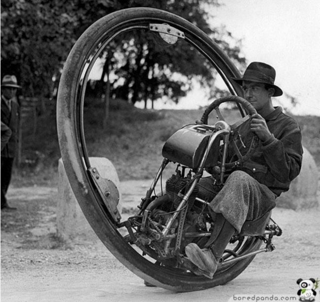
The One Wheel Motorcycle, capable of reaching a top speed of 93 mph. (1931)
